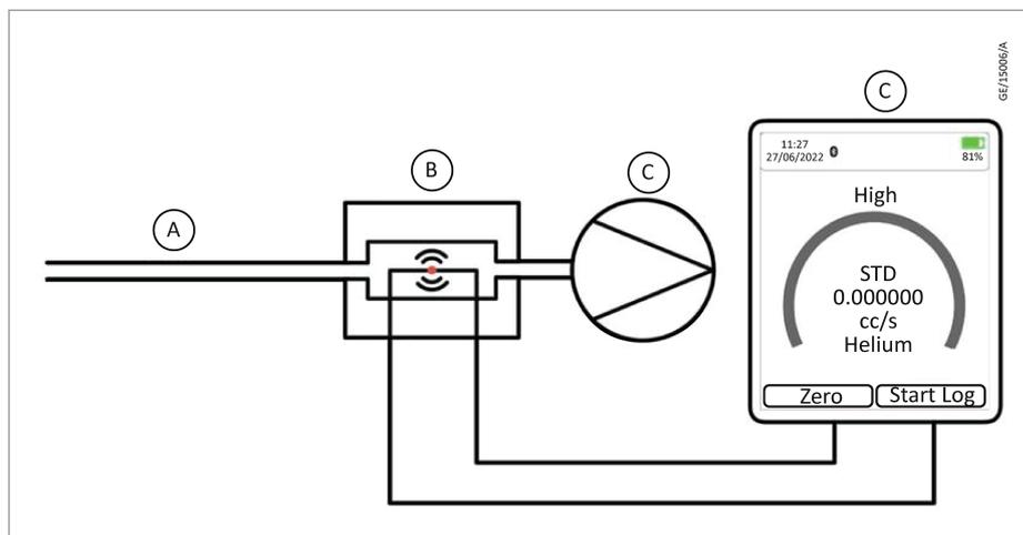
When gases with different thermal qualities pass through the chamber, the amount of heat being transmitted changes. These changes are measured and used to calculate a display reading for leak rates or gas concentrations.
