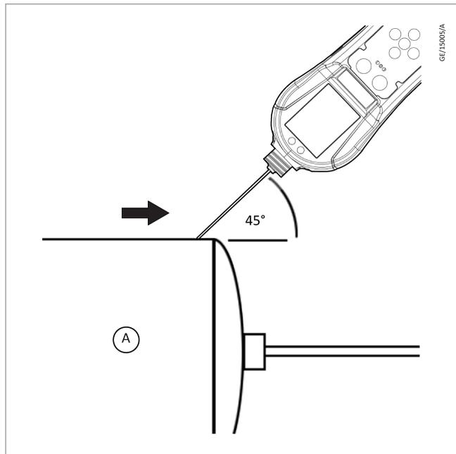
The probe cover can be removed to allow better access to restricted areas, if the probe cover is removed the following points should be noted: -
