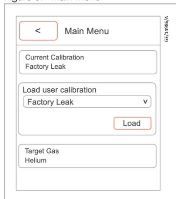
The current calibration button provides you with information on when the instrument was last calibrated, what gas was used, what the concentration was and what the mV response was.
