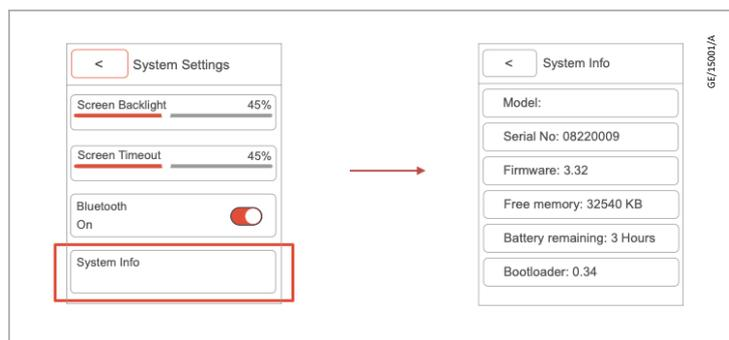
Provides you with: Phoenix Mobilis Ultra model, serial number, firmware, memory, battery remaining and bootloader.
