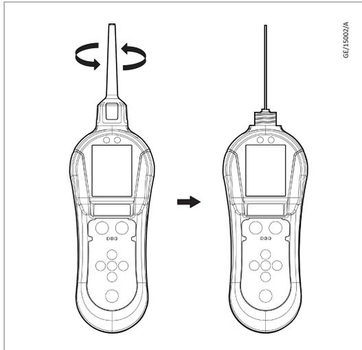
Some applications might require a longer probe to gain access to pneumatic joints and seams. The instrument is supplied with a 20 cm flexible probe that can be changed by the user. To change the probes, following the below steps:
