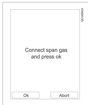
6. Once the instrument has stabilised, the calibration will finish. To confirm calibration, press ok, again, you can abort at this stage if required. The calibration will then save to the instrument. This calibration will automatically be added to the user load list.
