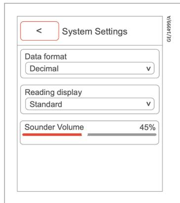
Allows you to adjust the alarm volume of the instrument (0-100).
