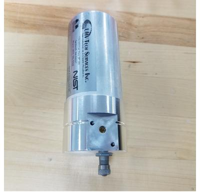
Once they get it back they need to install it and then go into the menu and press menu/settings/vacuum setting/ leak rate internal/ yes to change. Enter the new value and save. Turn the unit on and let it run for 20 minutes. Run a cal by pressing cal. The old cal factor and new should not be that different. They should also spray some helium around the V7 valve once finished to make sure it is leak tight.
