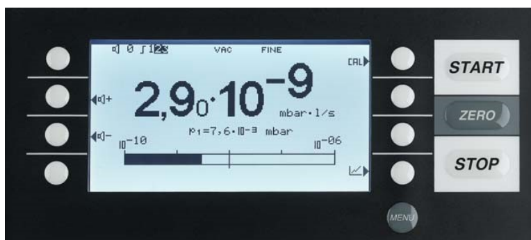
Figure 10 Display: measurement mode with bar graph
